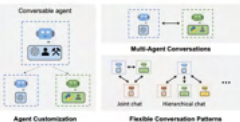
Figure 1: AutoGen enables complex LLM-based workflows using multi-agent conversations. (Left) Multiple agents are customizable and can be based on LLMs, tools, humans and even a combination of them. (Top-right) Agents can converse to solve tasks. (Bottom-right) The framework supports many additional complex conversation patterns.
